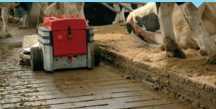
Manure is pushed through the openings of the slatted floors.
